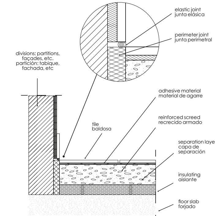
DETAIL OF PERIMETER JOINT WITH SEALANT | DETALLE DE JUNTA PERIMETRAL CON SELLANTE
