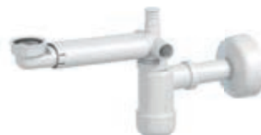
Furniture waste trap Suitable in combination with a low waste plug. The space in the bottom drawer of the furniture is not limited by the waste trap body. The drawer inside stays intact and holds larger items. Order No. X01612
