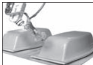
Moulding reinforcement Reinforcement of the moulding by resin with addition of fibreglass or polyurethane foam PU.
